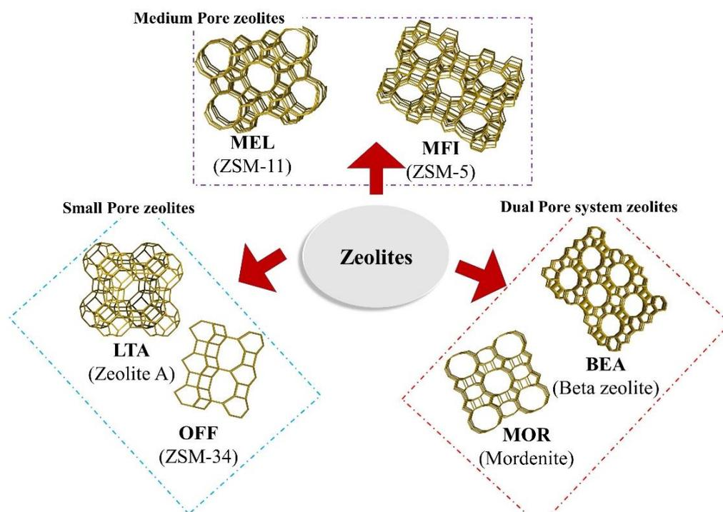
**Figure 5.** Classification of zeolites according to the pore system. Medium pore zeolites: MEL (Zeolite Socony Mobil-eleven, ZSM-11) and MFI (Zeolite Socony Mobil-five, ZSM-5). Dual pore system zeolites: BEA (Zeolite Beta polymorph A) and MOR (Mordenite). Small pore zeolites: LTA (Linde Type A), Zeolite A, OFF (Offretite) and ZSM-34 (Zeolite Socony Mobil-thirty-four).
