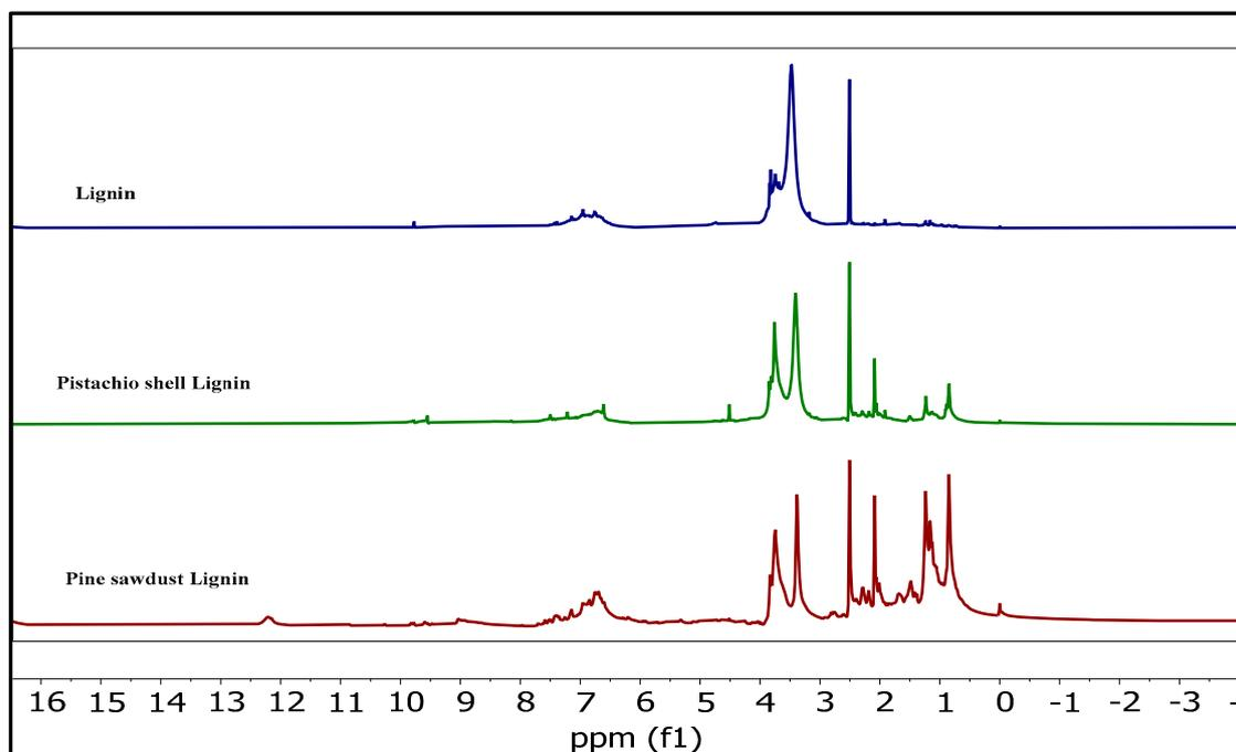
**Figure 4.**  $^1\text{H}$ -NMR spectrum of extracted lignin from pine sawdust and pistachio shells compared with commercial lignin.
