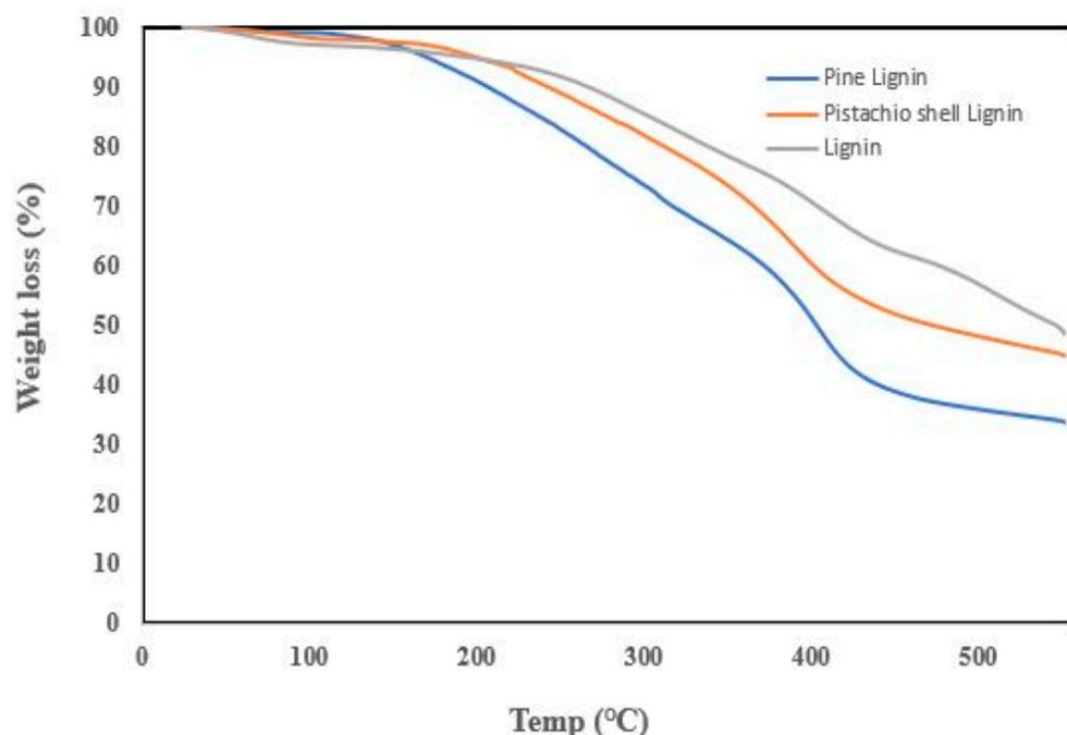
**Figure 5.** TGA plots of lignin from pistachio shells, pine sawdust, and commercial lignin obtained under nitrogen atmosphere at 10 °C/min.
