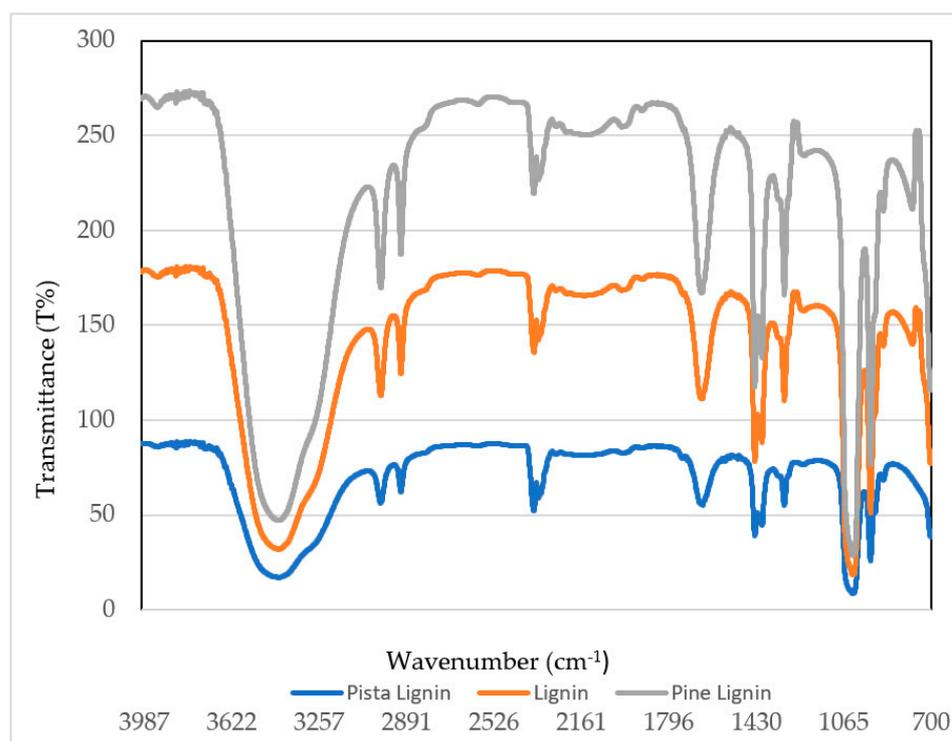
**Figure 3.** FTIR spectrum of extracted lignin from the pistachio shell and pine sawdust biomass and compared with commercial lignin.
