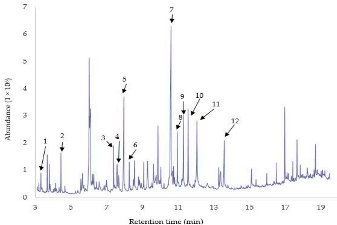
**Figure 6.** GC-MS total ion chromatogram of phenolic monomers from pine sawdust lignin.
