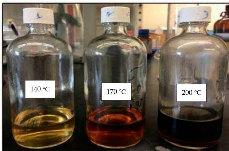
**Figure 2.** Extraction of lignin from the pine sawdust biomass at different temperatures.
