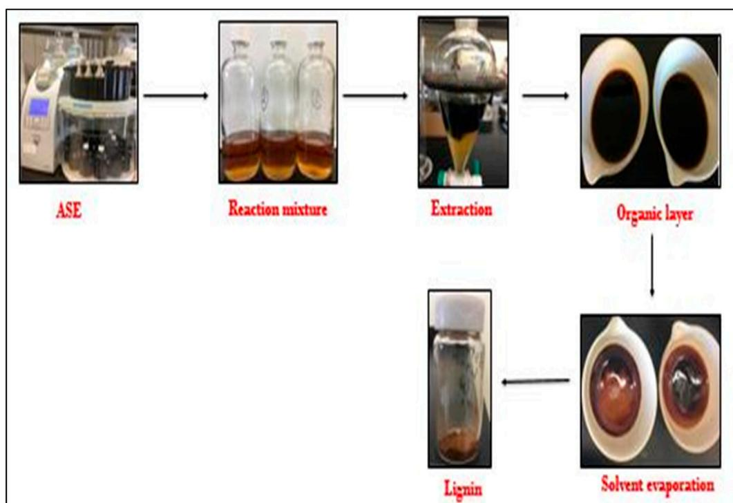
**Figure 1.** Extraction of lignin from the biomass using accelerated solvent extraction (ASE).
