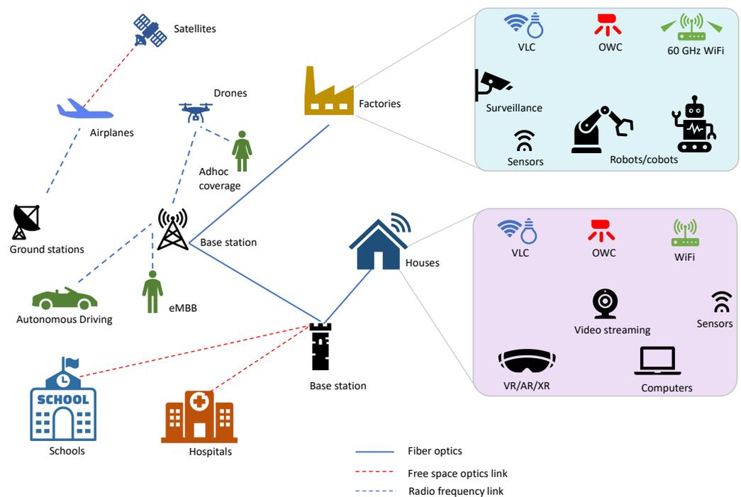
**Figure 1.** Components of the 6G ecosystem.
