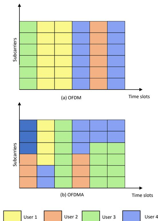
**Figure 3.** (a) OFDM systems allocate all the subcarriers to a single user; (b) OFDMA systems can allocate sets of subcarriers to different users.
