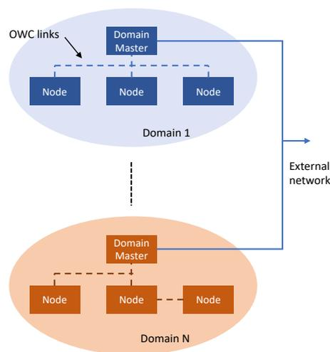
**Figure 8.** Network architecture reference model of G.vlc.
