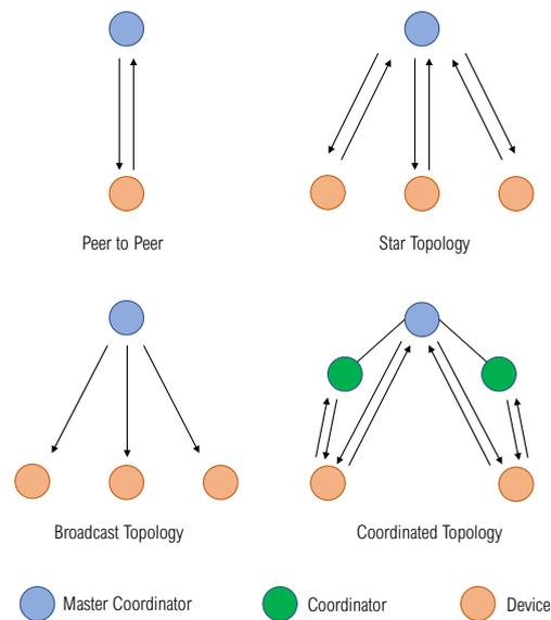
**Figure 7.** Network topologies supported in IEEE 802.15.13 standard.
