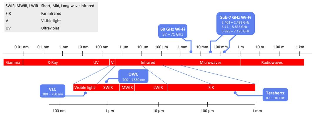
Figure 2. Positioning of the communication technologies in the electromagnetic spectrum.
