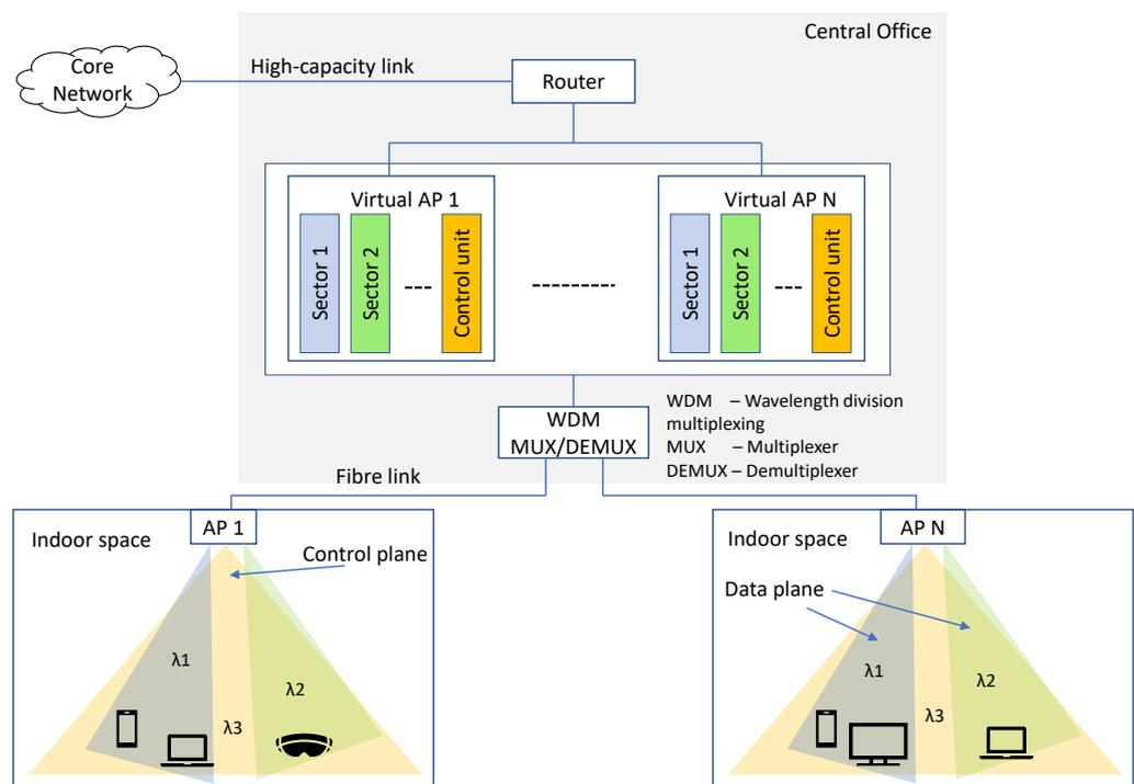
Figure 10. Split-plane architecture for OWC.
