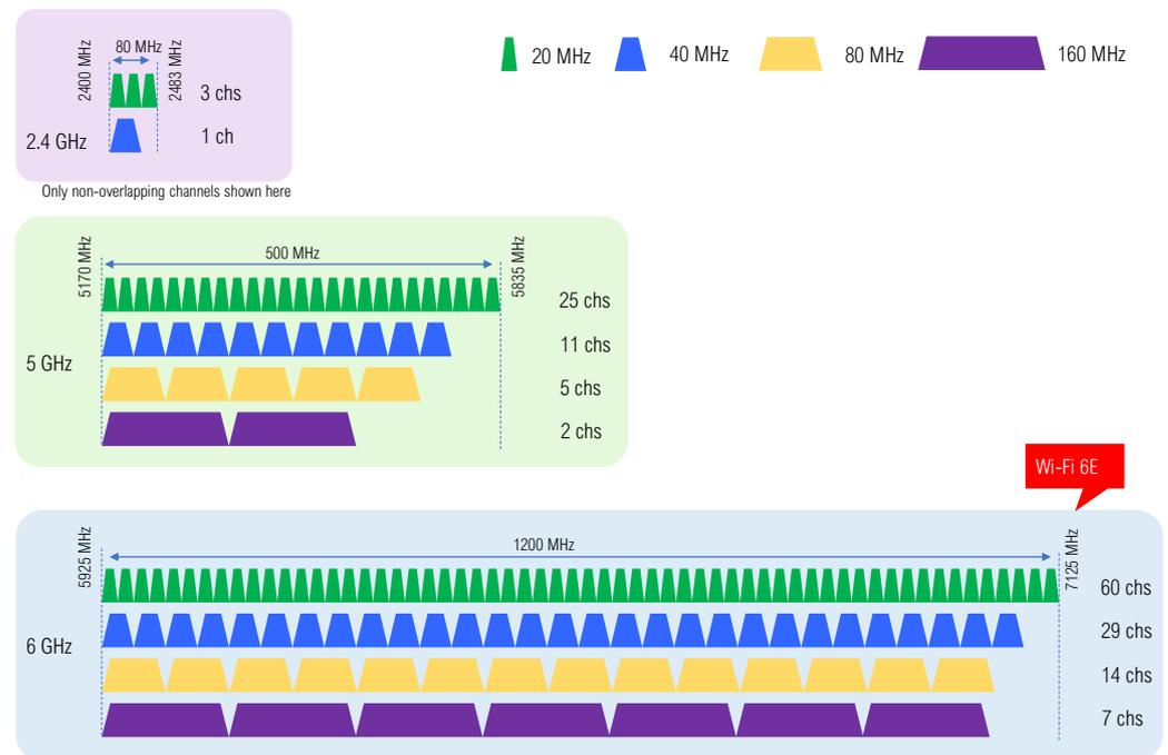
**Figure 4.** Channelization of sub-7 GHz WiFi standards.
