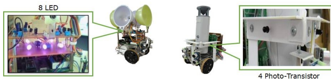
Figure 11. New devices for signal emission and detection. For the chasing robot, 8 LEDs are used, and on the fleeing robot, 4 photo-transistors are used.
