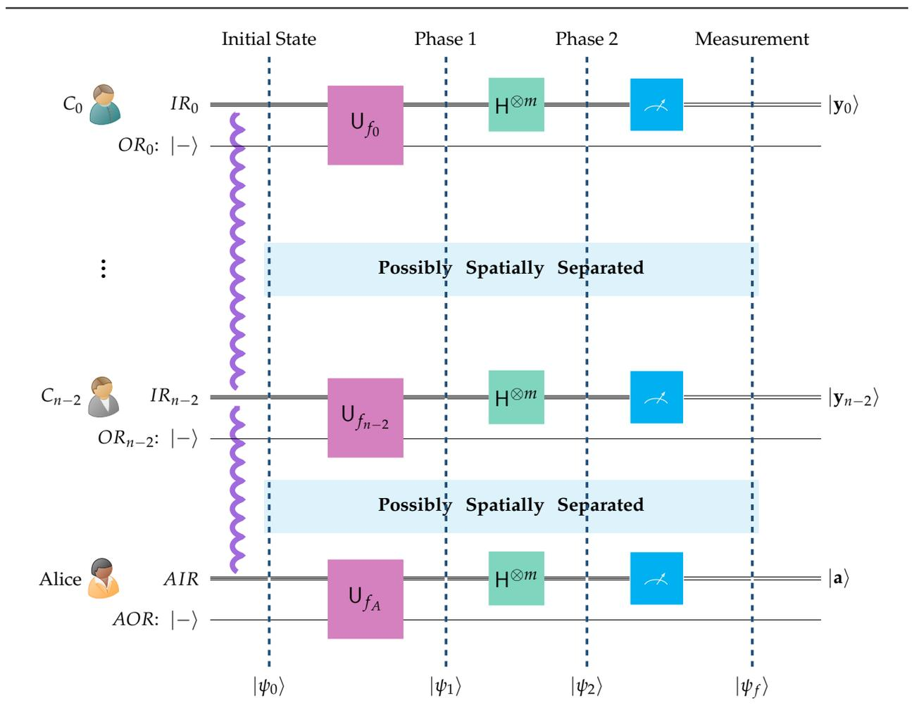
**Figure 4.** The above figure shows the composite quantum circuit used by the dining cryptographers, composed of the individual local circuits Alice and her colleagues possess. Even if these local circuits are spatially separated, they still constitute one composite system because they are linked due to entanglement. The state vectors  $|\psi_0\rangle$ ,  $|\psi_1\rangle$ ,  $|\psi_2\rangle$ , and  $|\psi_f\rangle$  describe the evolution of this composite system.
