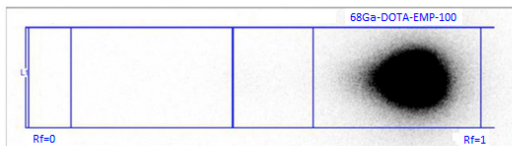
Figure 3. Radio-TLC chromatogram of [^{68}\text{Ga}]\text{Ga-DOTA-EMP-100} .
