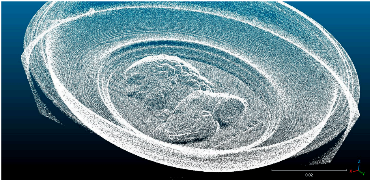
Figure 47. Point cloud of the medallion measured using the AS1 scanner.
