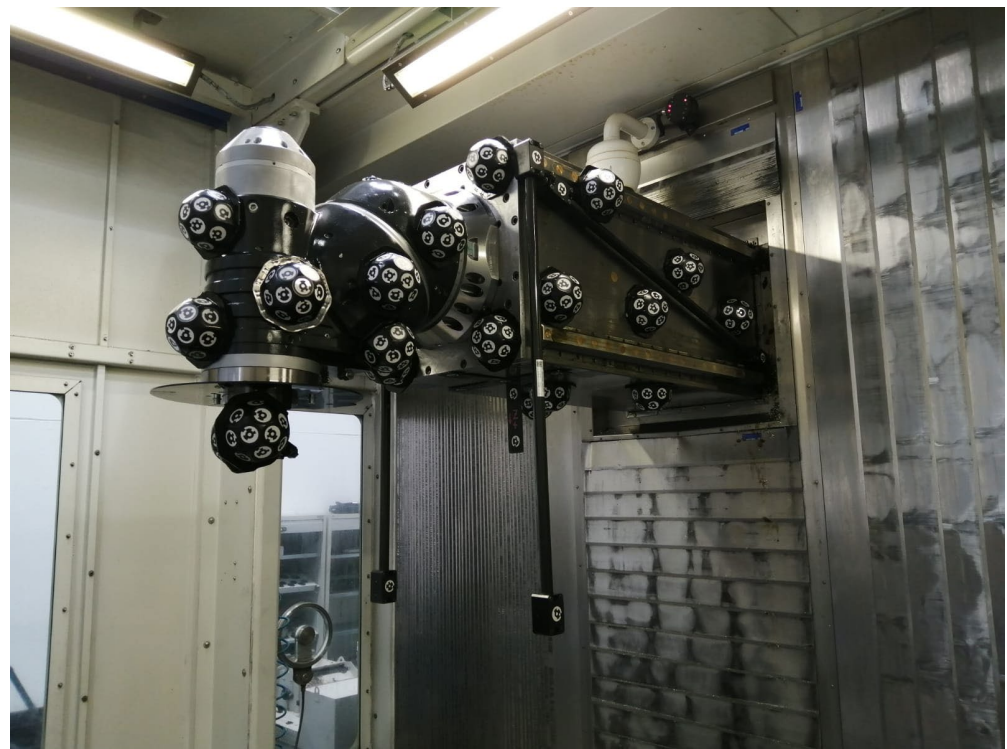
Figure 4. VSET markers across the Soraluce machine for static measurement.
