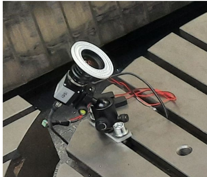
Figure 2. One of the four tracking system cameras deployed in the milling machine workspace.
