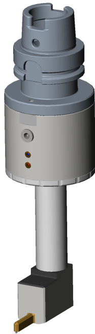
Figure 4. CAD model of machine tool-integrated roughness measurement system.
