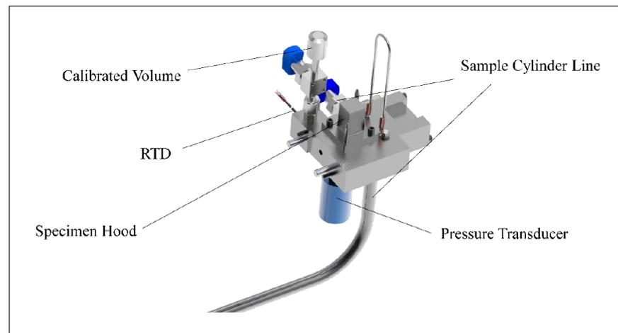
**Figure 1.** Concept drawing of the SATGAS module.
