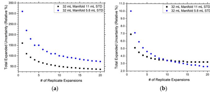
**Figure 2.** The expanded uncertainty in relative percent vs. the number (#) of replicate expansions used to calculate the averaged volume for (a) 0.07 mL and (b) 2.5 mL rodlet volumes. Data from the 11.85 mL volume standard and the 5.807 mL volume standard are graphed together to illustrate the change in expanded uncertainty.
