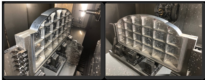
Figure 11. Manufacturing of MPQP test artefacts by NC machining operations.
