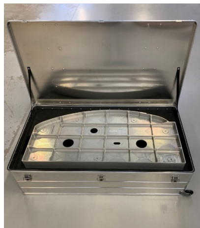
Figure 14. Each MPQP test artefact is securely stored in dedicated and marked aluminium containers/boxes. Every container/box can store a maximum of two MPQP artefacts.
