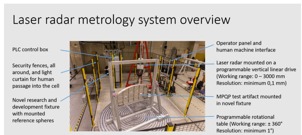
Figure 21. Principal construction of the laser radar measuring cell.
