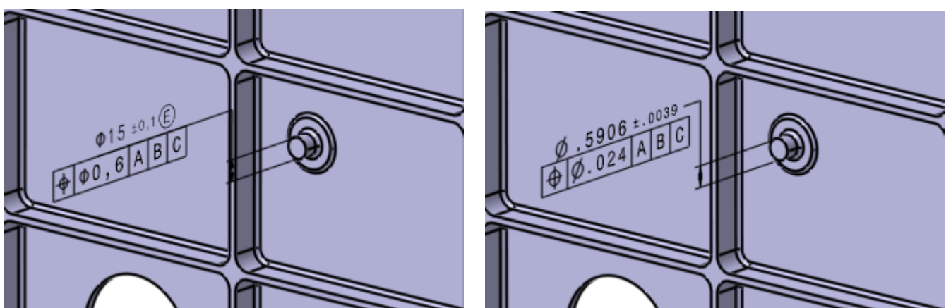
Figure A9. Pin specified in ISO model (left illustration) and Pin specified in ASME model (right illustration).
