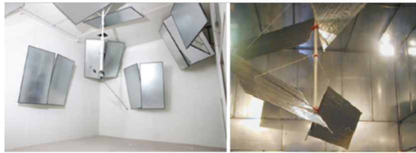
Figure 3. (Left) Diffusers in reverberation chamber (ETS Lindgren Company, Cedar Park, TX, USA) (Right) Stirrer in reverberation chamber (Ecotone Systems Pvt. Ltd., Greater Noida, Uttar Pradesh, India).
