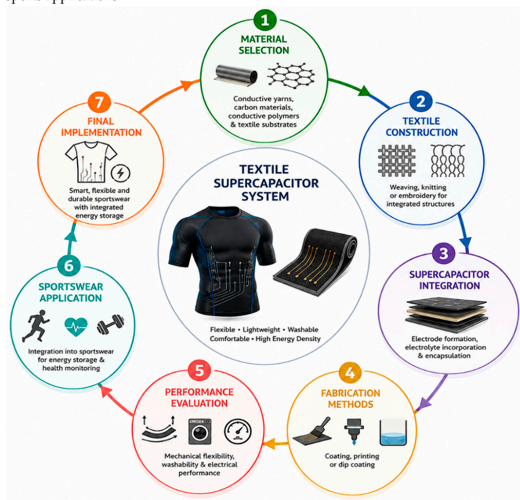
Figure 1. Comprehensive flow diagram for supercapacitor-based systems in sports e-textiles, including material selection, textile structure, integration process, fabrication methods, performance testing, and sportswear applications.
