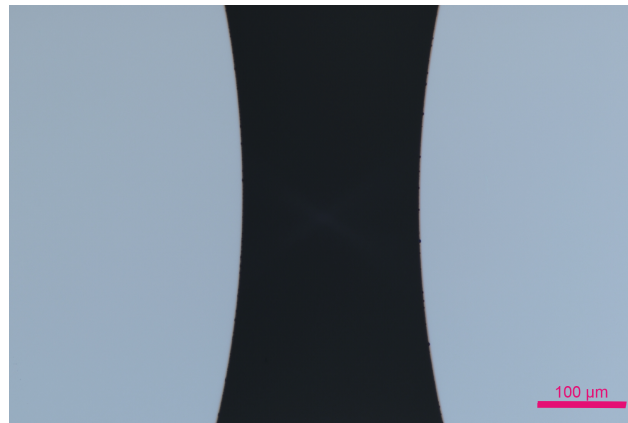
Figure 13. Microscope image of a 60/40/60 nm reflector stack before annealing.
