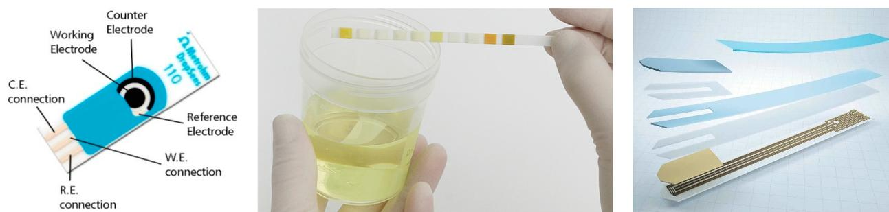
**Figure 1.** Conventional, reusable screen-printed thick-film sensor on ceramic from Metrohm DropSens [19] (**left**) semi-quantitative color changing urine test strips Combur-Test® from Roche Diagnostics [20] (**middle**) and laminated assembly of one-way blood sugar test strips [21] (**right**). Adapted and reprinted with permission from The American Diabetes Association. Copyright 2023 by the American Diabetes Association.
