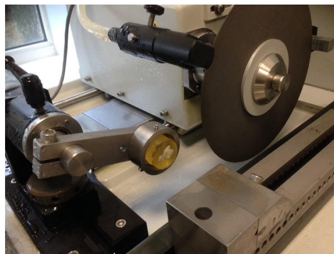
Figure 1. The process of forming a slice of a sample on a linear precision cutting machine.
