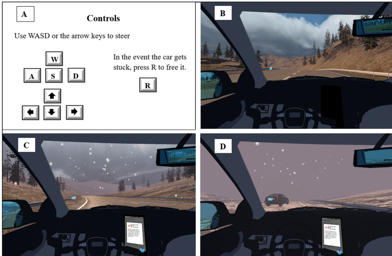
Figure 1. Browser-based snow-driving simulation environment and experimental scenarios. (A) Simulation control interface and keyboard interaction method; (B) baseline mountainous roadway environment before snowfall intensification; (C) moderate snowfall conditions with reduced visibility; and (D) intensified snow-driving conditions illustrating decreased visibility, snow accumulation, and environmental driving hazards [28].
