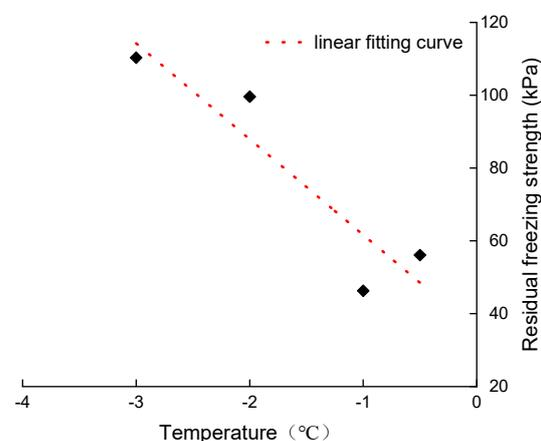
**Figure 8.** Residual freezing strength of thawing frozen soil-pile interface at different temperatures.
