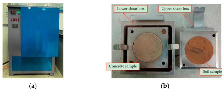
**Figure 3.** Testing equipments: (a) constant temperature environmental chamber; (b) direct shear test.
