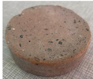
**Figure 2.** Concrete specimens.
