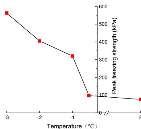
**Figure 7.** Peak freezing strength of thawing frozen soil-pile interface at different temperatures.
