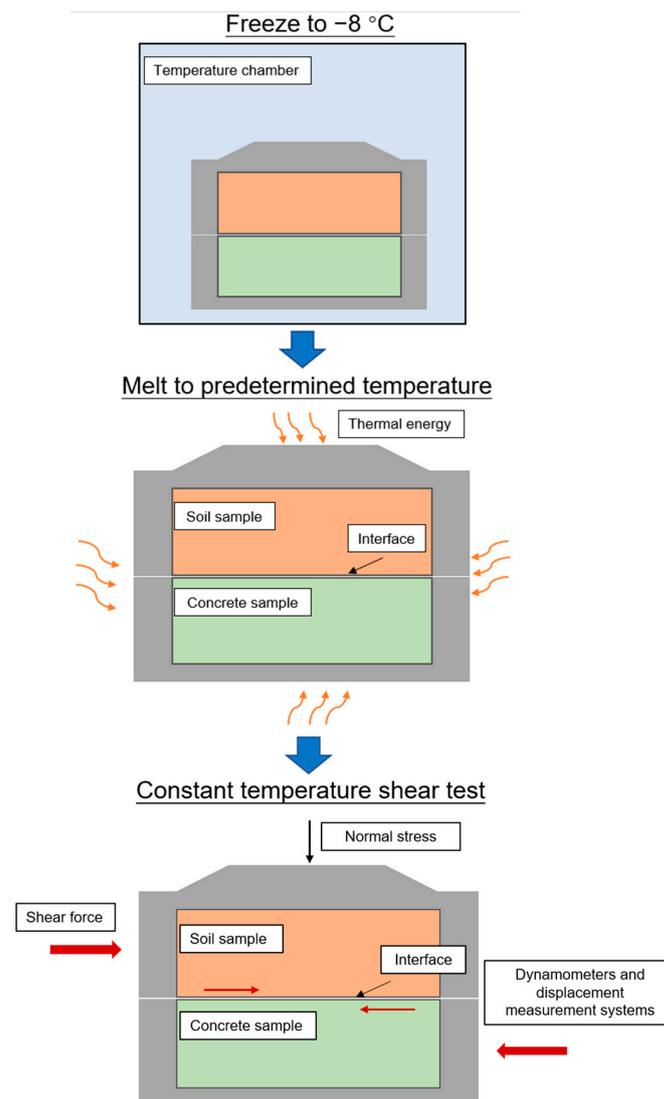
**Figure 4.** Schematic diagram of the shear test process.
