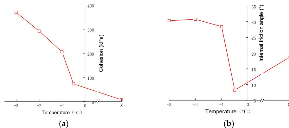
**Figure 9.** Temperature dependence of mechanical parameters of thawing frozen soil-concrete pile interface: (a) change in cohesion; (b) change in the internal friction angle.
