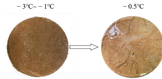
**Figure 6.** Shear surface characteristics of thawing frozen soil-concrete at different temperatures.
