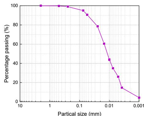
**Figure 1.** Gradation curve of the soil sample.
