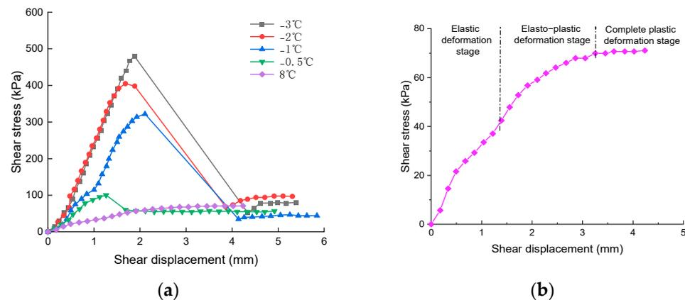
**Figure 5.** Shear stress–displacement curves at the soil–concrete pile interface at different shear temperatures: (a) overall diagram; (b) 8 °C shear temperature.
