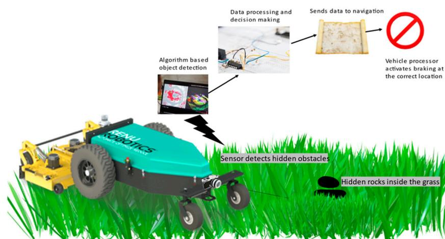
**Figure 1.** Concept of self-driving vehicle in the field.
