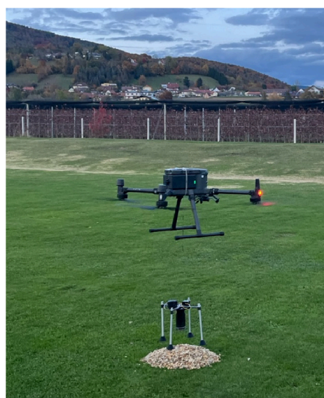
Figure 16. Sampling gravel with the screw pipe.
