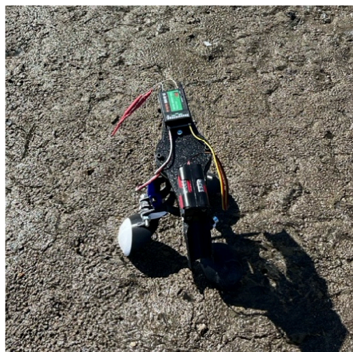
Figure 12. Application of the grab arm on SP6.
