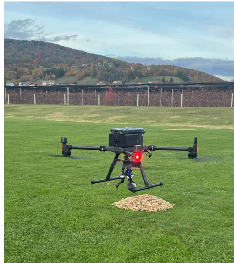
Figure 15. Sampling gravel with the grab arm.
