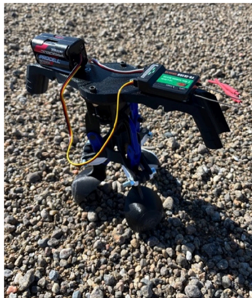
Figure 9. Application of the grab arm on SP3.
