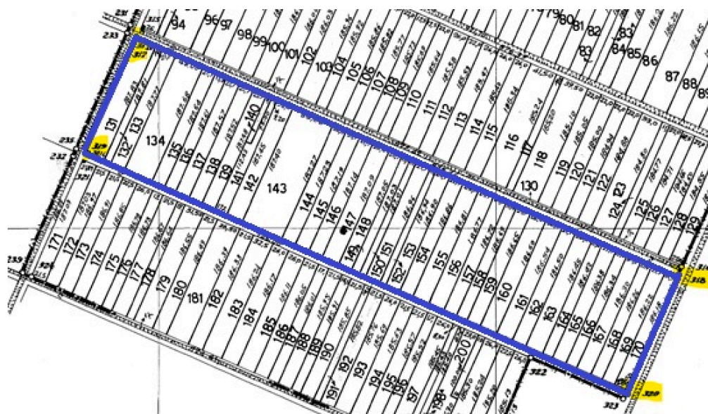
Figure 3. Rural parcel transformed from NVGRD to HGRS87 (Nea Amisos village, Greece). Boundary coordinates originate from a New Version of the Greek Datum plan and were transformed to HGRS87 (EPSG:2100). The parcel boundary is highlighted; the underlying plan is reproduced from Hellenic Cadastre records.
