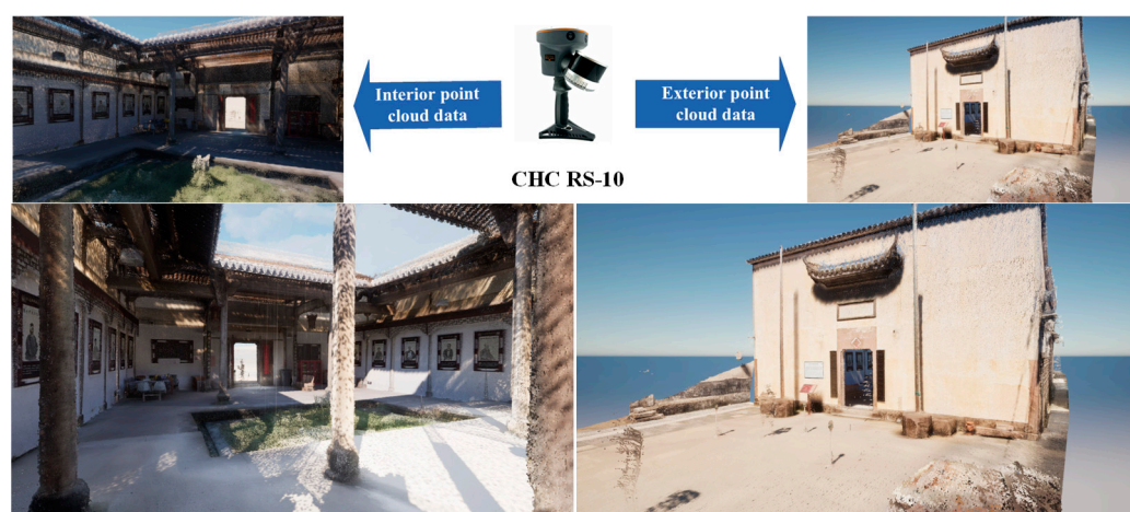
Figure 4. Handheld SLAM and its Scene Shooting Example.
