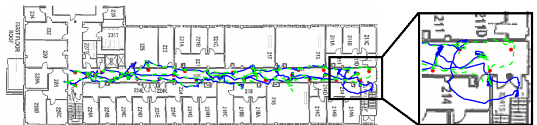
Figure 13. UWB trajectory in an indoor building hallway with trajectory estimated without calibration shown as blue solid line and with considered calibration model as green dashed line (Source: [102]).
