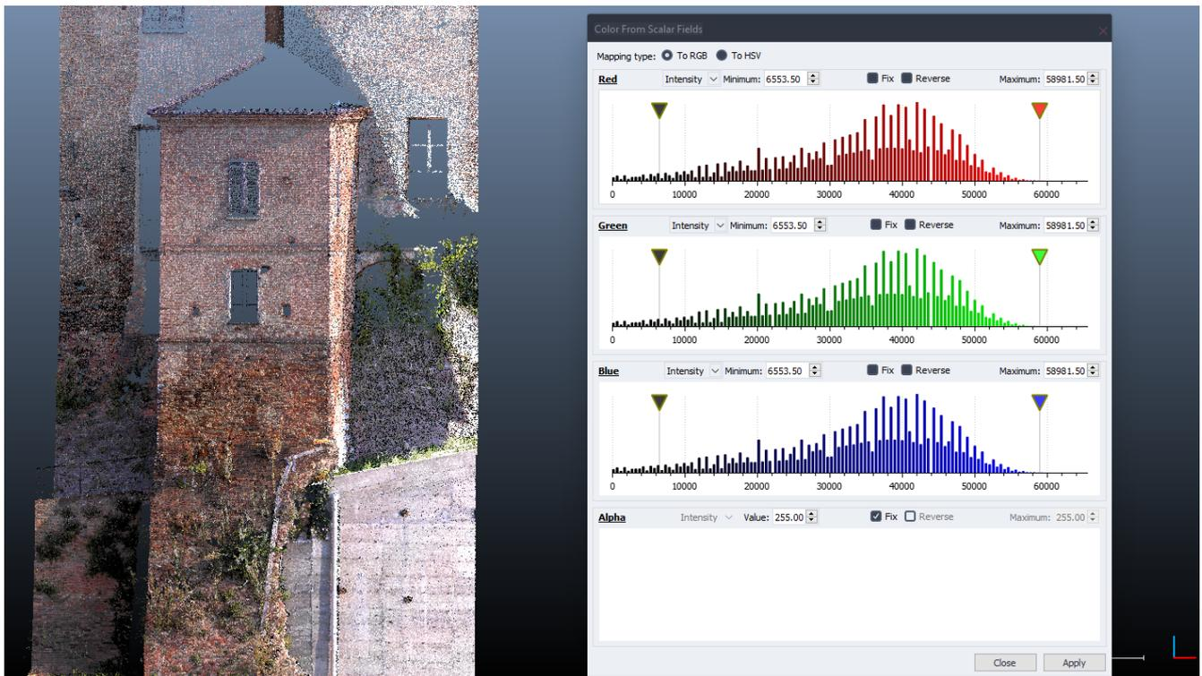
**Figure 31.** Radiometric values and red, green, and blue spectrums related to the TLS point clouds of the entrance tower.
