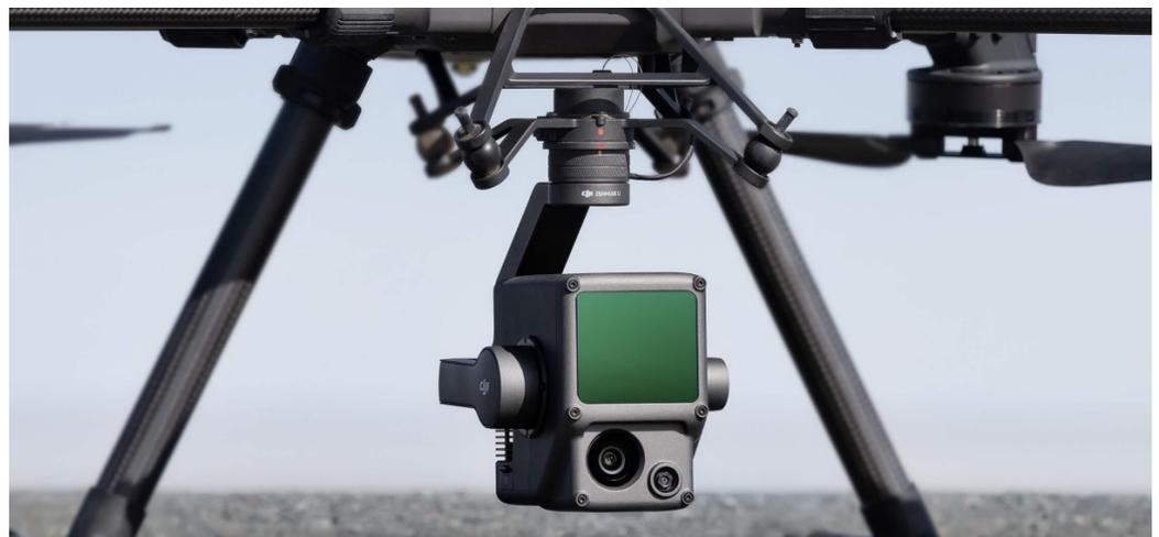
**Figure 2.** Zenmuse L1 LiDAR sensor, anchored to a gimbal and a DJI Matrice 300 RTK drone (image from [www.dji.com](http://www.dji.com) accessed on 10 July 2022).
