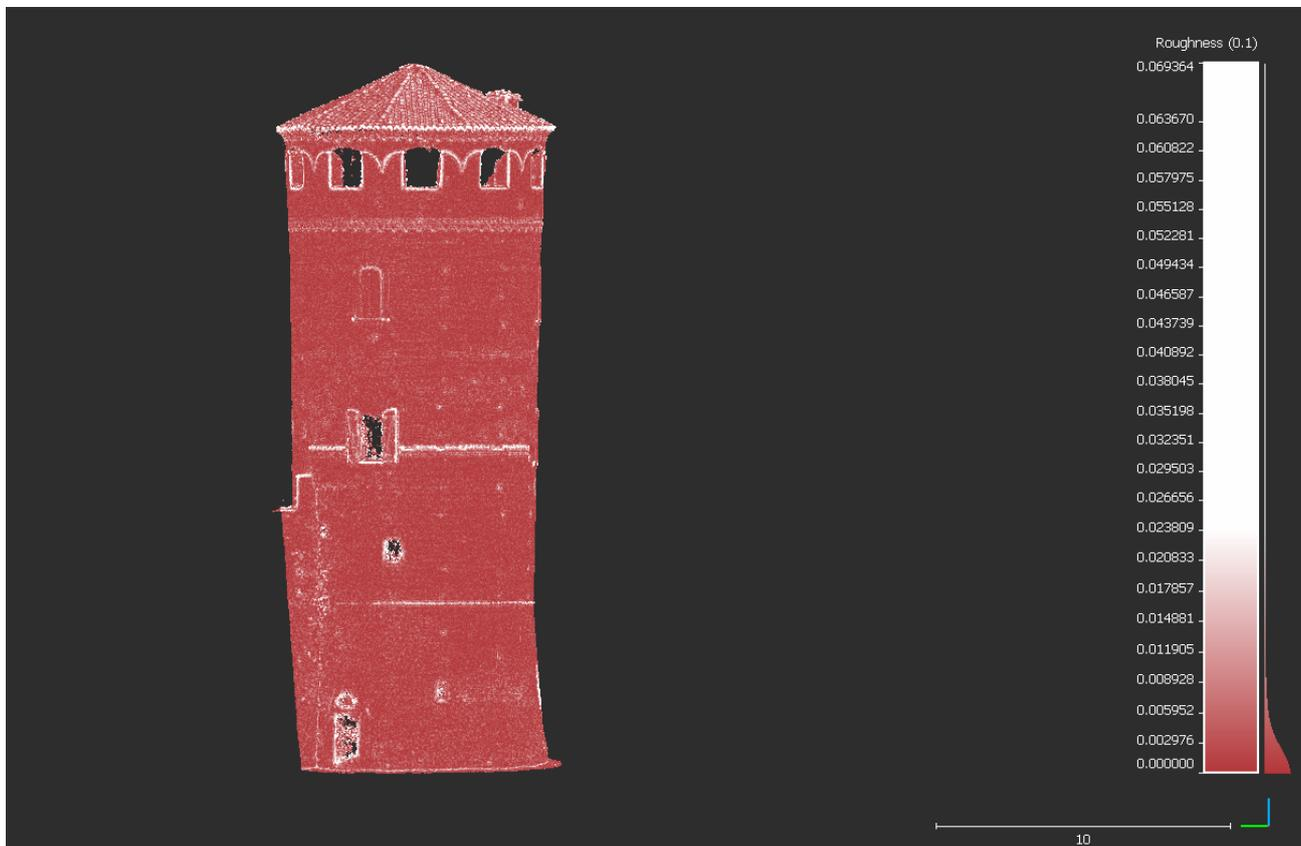
Figure 28. Roughness analysis of the photogrammetric data: RMSe 0.006 m; standard deviation 0.005 m. White points are related to roughness and noise record.
