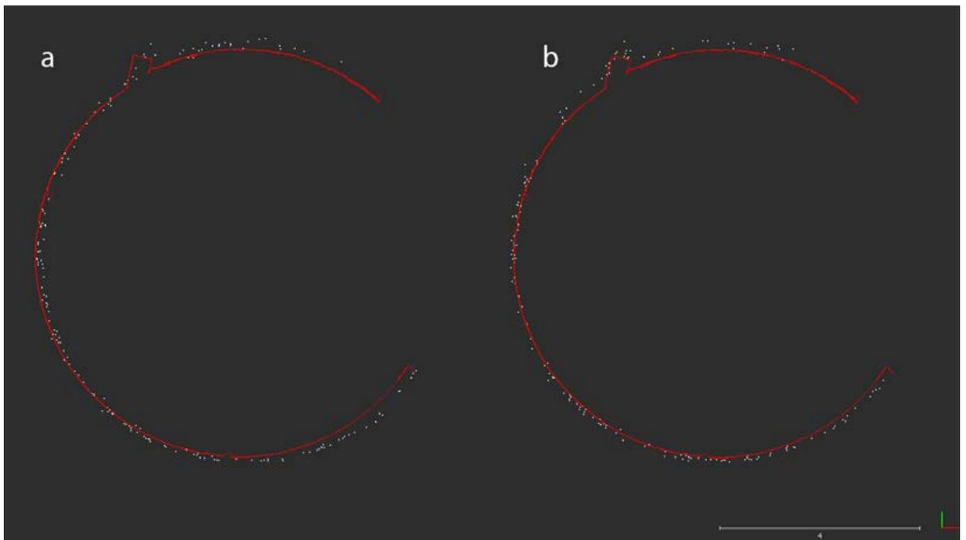
**Figure 14.** Section on z axis. ICP analysis on L1 data (white—aligned) and SX10 (red—static reference): (a) before the alignment; (b) after the alignment. L1 points dimension 2 pixels; SX10 points 1 pixel.
