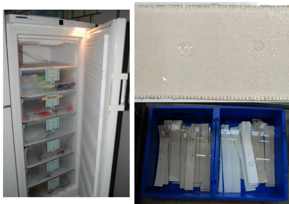
**Figure 3.** Left: cold chamber, top right: glass-PTFE surface after freeze cycle, and bottom right: thaw cycle.
