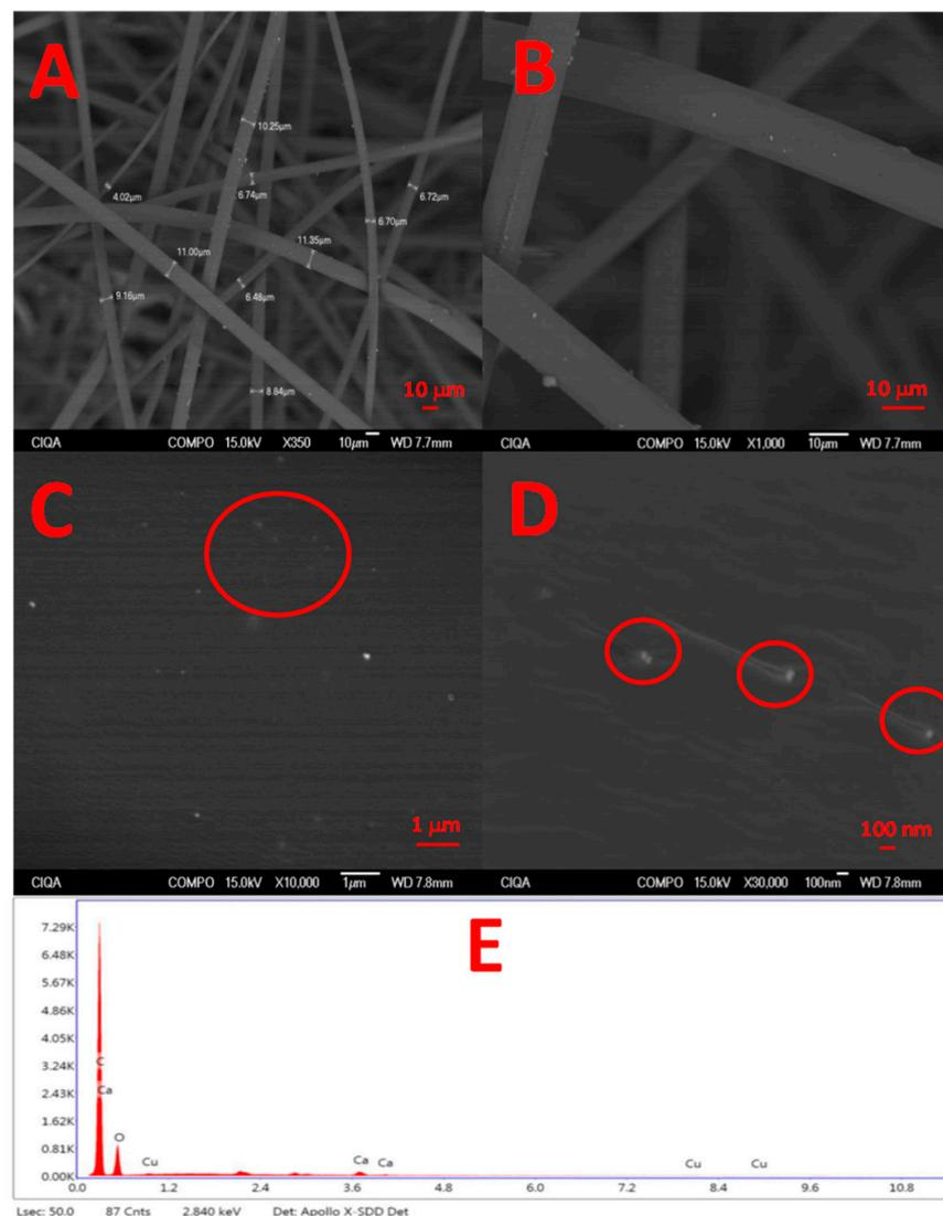
**Figure 5.** SEM images for the NWF of PET/CuNP (0.5% *w/w*) sample at different magnifications. (A) 350 $\times$ , (B) 1000 $\times$ , (C) 10,000 $\times$  and (D) 30,000 $\times$ , and (E) elemental analysis of the sample.
