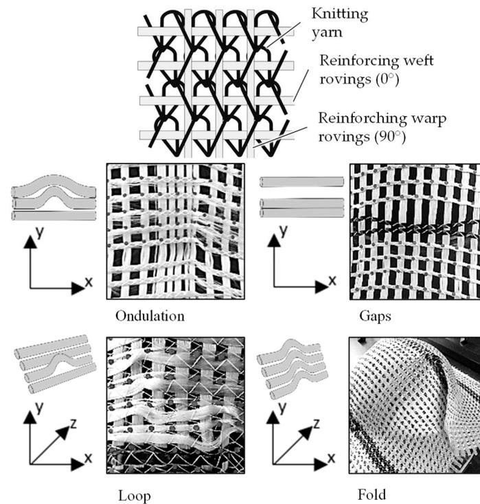
Figure 6. Drape effects occurring in open-meshed textile reinforcements.
