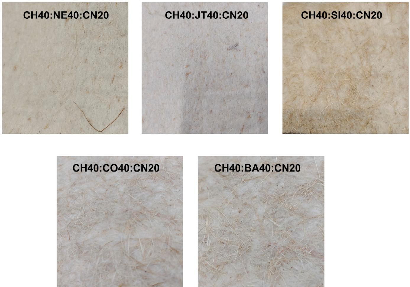
**Figure 1.** Photos of different nonwoven fabric produced from the needle punching machine.
