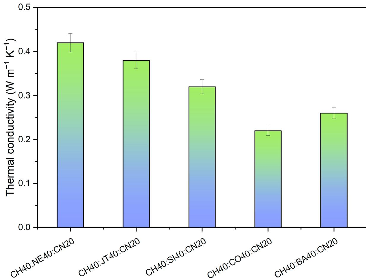
**Figure 8.** Influence of blend proportion on thermal conductivity.
