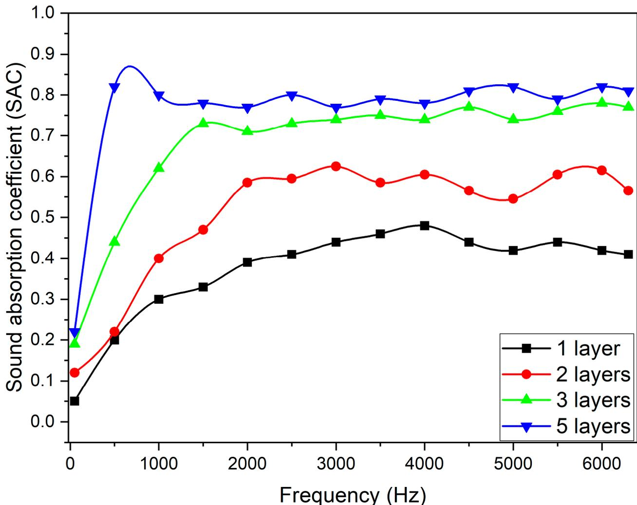
**Figure 4.** The sound absorption coefficient of the CH40:NE40:CN20 nonwoven fabric and the influence of the number of layers.
