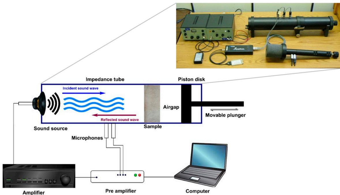
**Figure 2.** Experimental setup for acoustical characterization.
