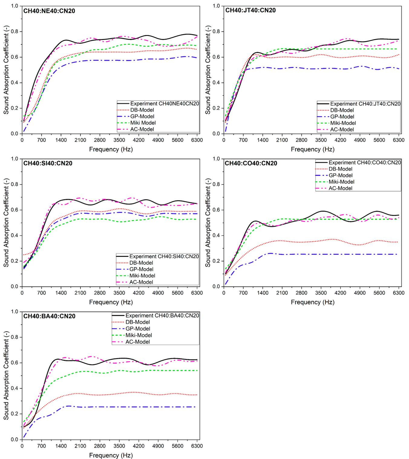
**Figure 6.** Predicted and experimental sound absorption coefficient values of the produced nonwoven fabrics with different blend proportions.
