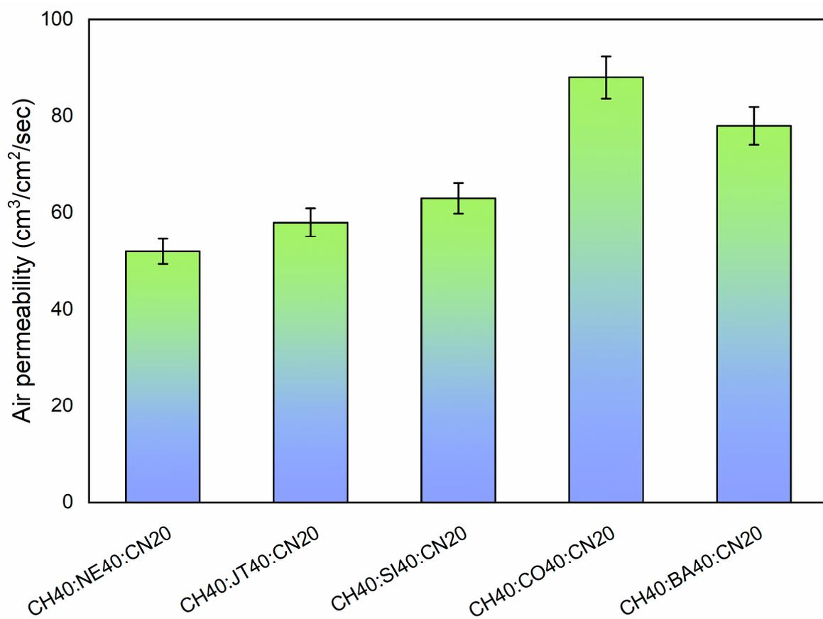
Figure 9. Influence of blend proportion on air permeability of nonwoven fabrics.
