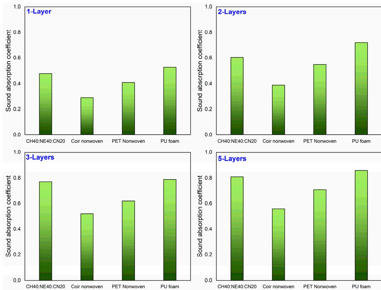
**Figure 7.** Results of the sound absorption coefficient on the CH40:NE40:CN20 nonwoven fabrics with commercially available sound absorption materials like coir nonwoven [60], PET nonwoven and PU foam [61].
