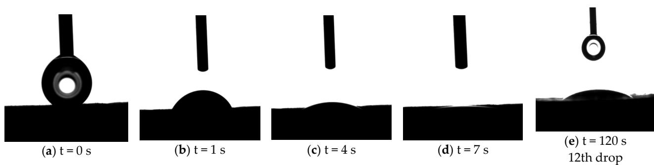
**Figure 10.** Water contact angles of leather coated by composite xerogels at different time intervals.
