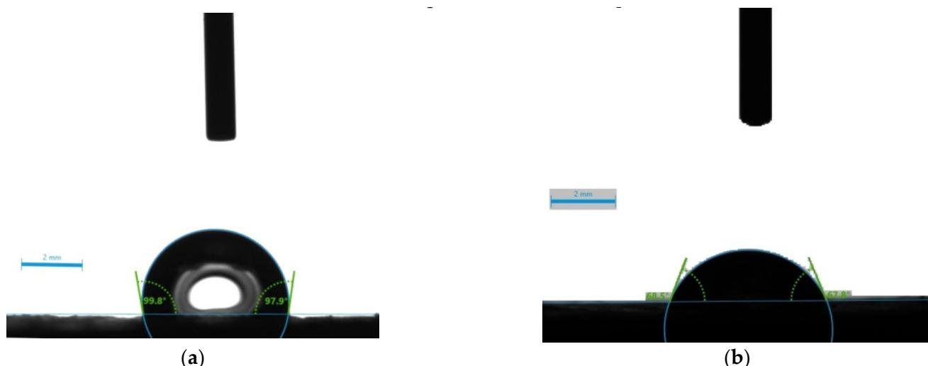
**Figure 9.** Water contact angles of raw leather (a) and leather modified by PEI-Ag Nps solution (b).
