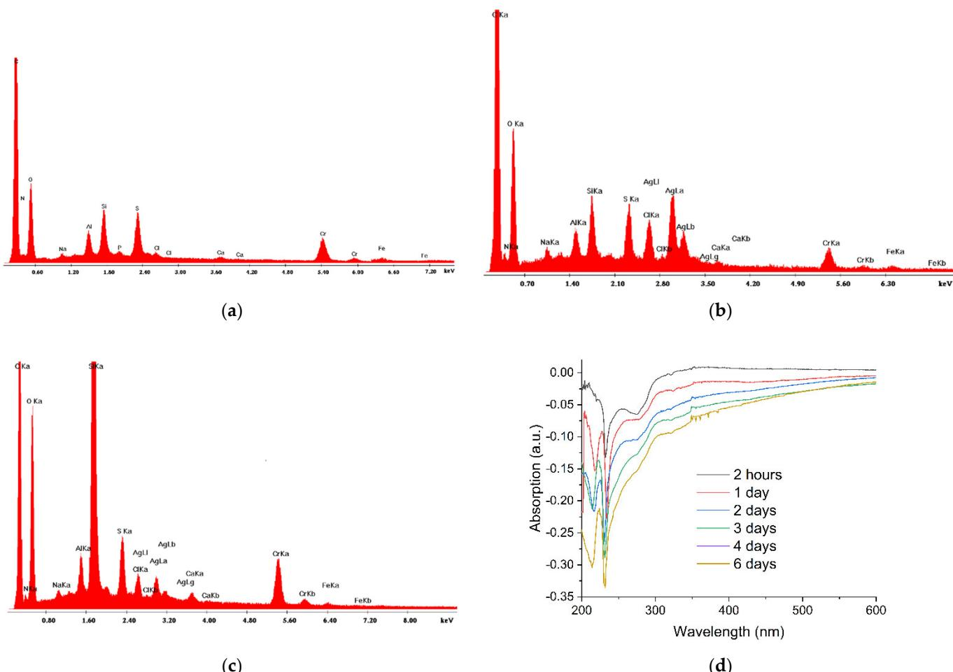
**Figure 5.** Energy-dispersive X-ray spectra of: (a) untreated leather; (b) leather wetted with PEI-Ag Nps; (c) leather coated by silica-PEI-Ag Nps composite xerogel; (d) UV-Vis spectra of the supernatant solutions of leathers coated with composite xerogels at different time intervals. The respective supernatants of untreated leathers are used as controls.
