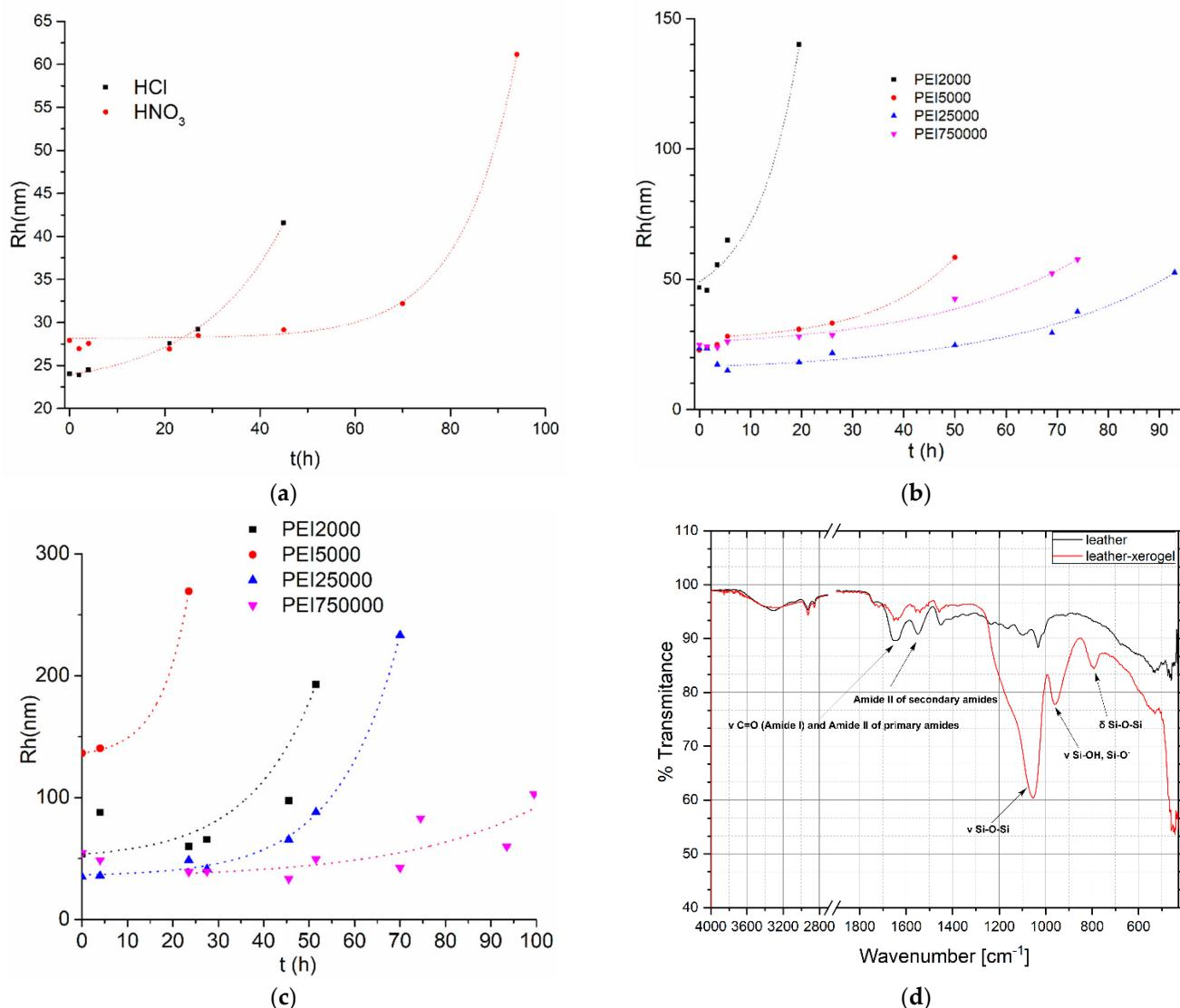
**Figure 3.** Size of agglomerates formed during the gelation process: **(a)** PEI 750,000 with tetra ethoxy silane hydrolyzed by HCl or HNO<sub>3</sub>, **(b)** Si(OH)<sub>4</sub>-PEI, and **(c)** Ag Nps-Si(OH)<sub>4</sub>-PEI-solutions as a function of time. **(d)** IR spectra of uncoated leather (black) and a sample coated with silica-PEI 25,000-Ag Nps xerogel (red), exhibiting the characteristic collagen and silica bands (v stretching, δ bending).
