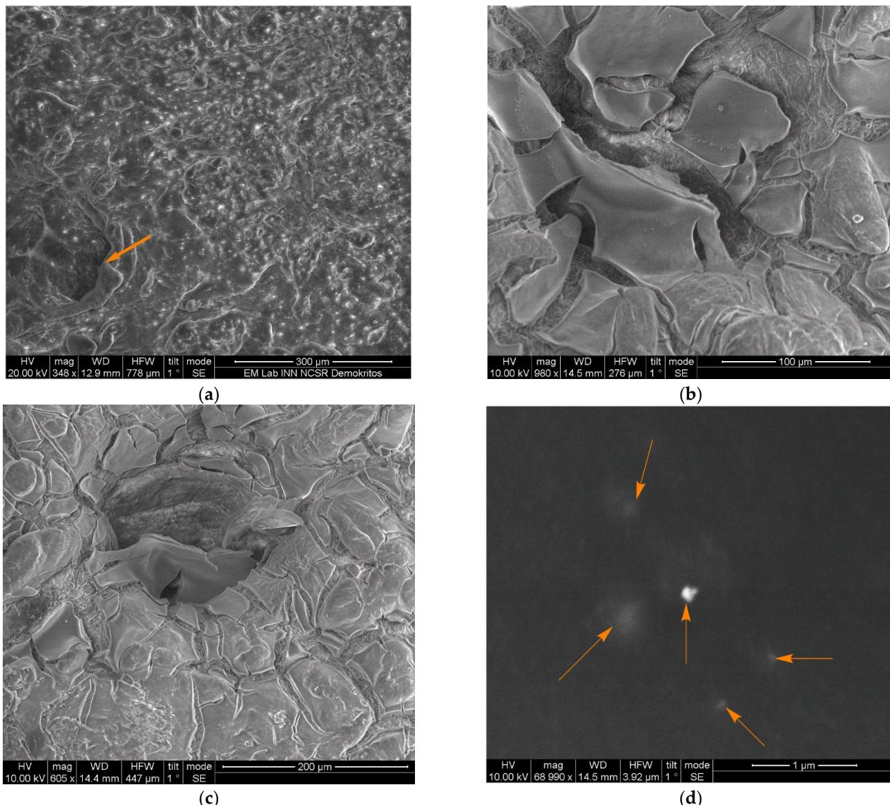
**Figure 4.** (a) SEM micrograph of uncoated leather and a pore (orange arrow); (b) SEM micrograph of leather coated in a single stage; (c) SEM micrograph coated in multiple stages indicating the penetration of the xerogel into the leather pores; (d) Ag nanoparticles incorporated into the xerogels (orange arrows).
