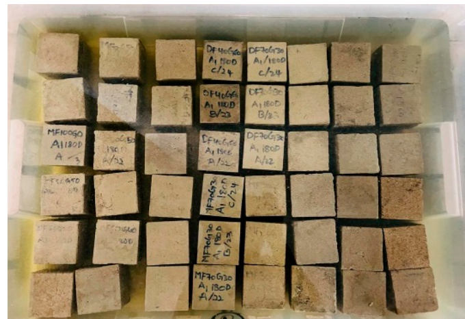
Figure 3. Mortar cubes immersed in hydrochloric acid.
