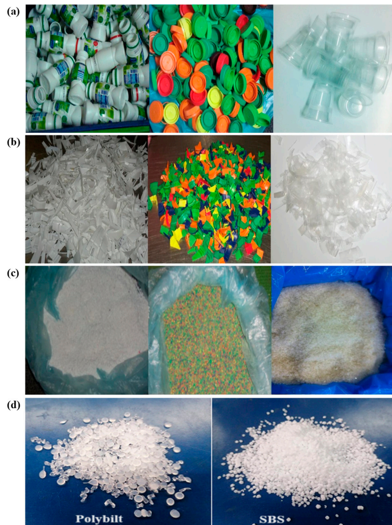
Figure 2. Polymers used for this study: (a) recycled plastic waste, (b) pre-shredding, (c) post-shredding, (d) commercial polymers ("B" and "S").
