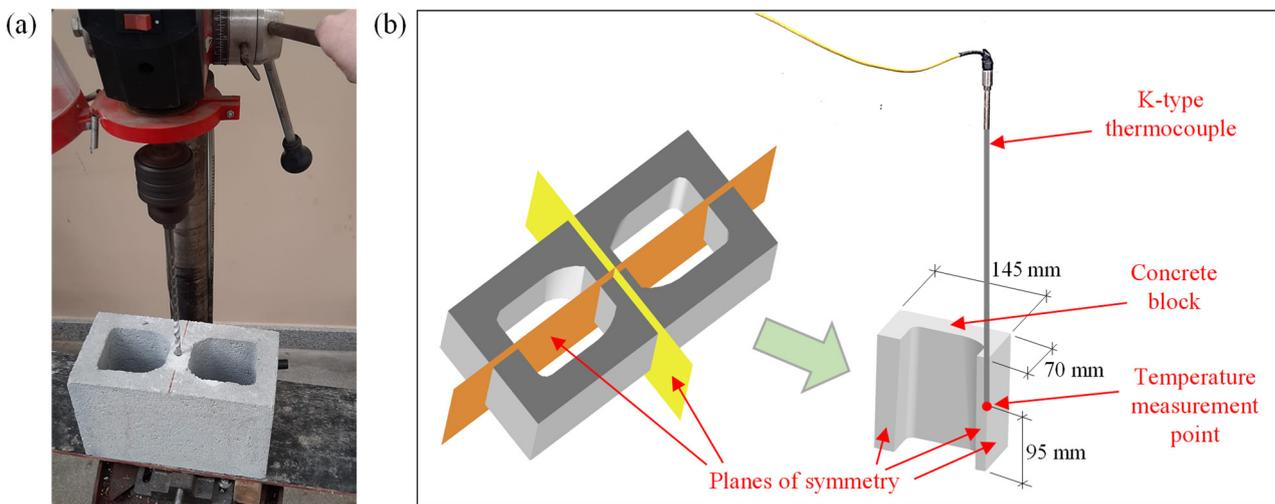
**Figure 1.** Hole drilled in the concrete blocks (a) and position and dimensions of the hole (b).
