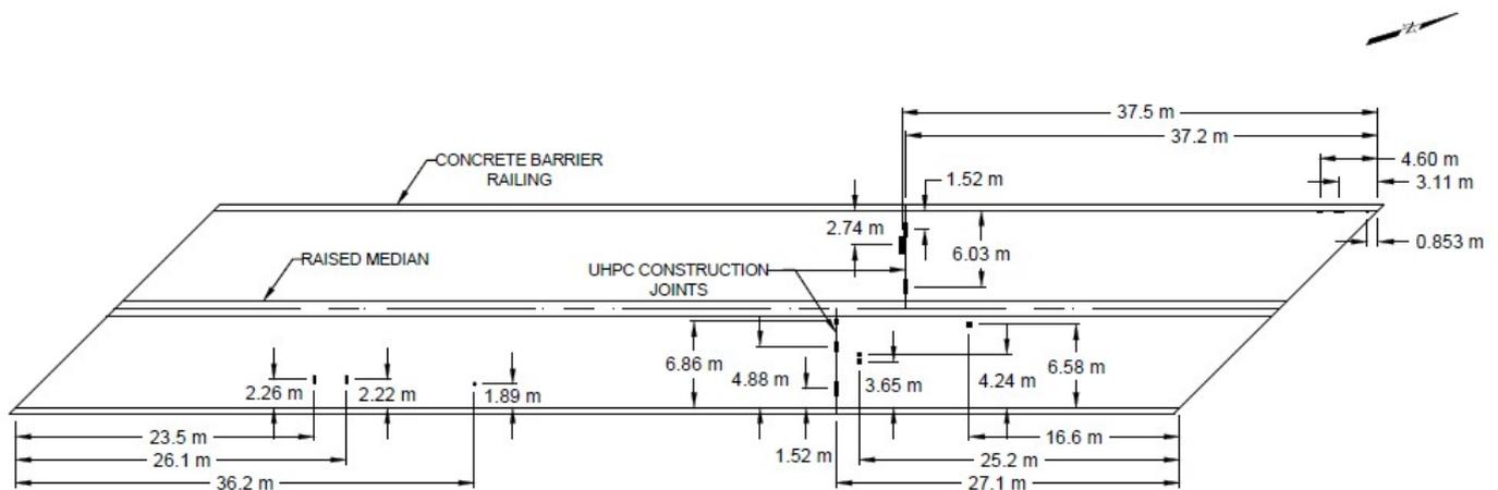
Figure 14. Potential delaminated areas identified on bridge no. 7032.
