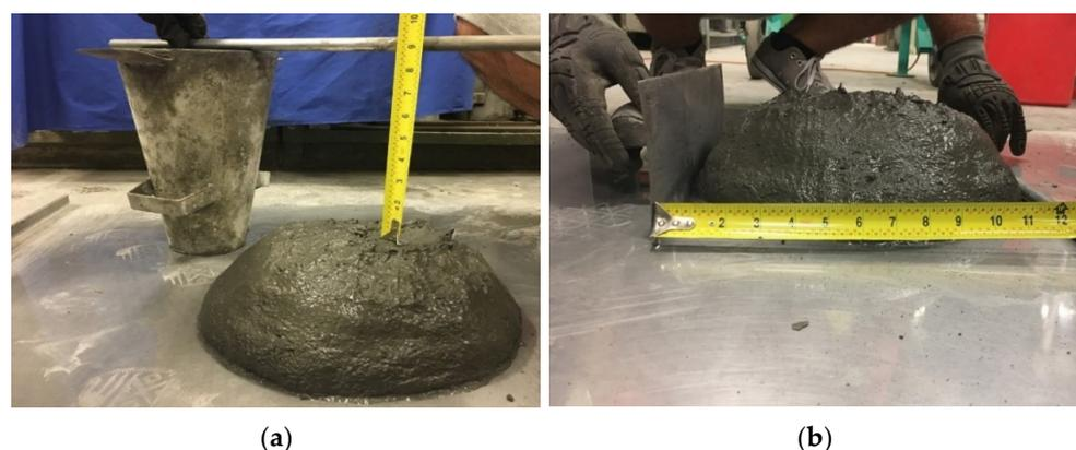
**Figure 8.** UHPC (a) slump and (b) slump-flow testing.
