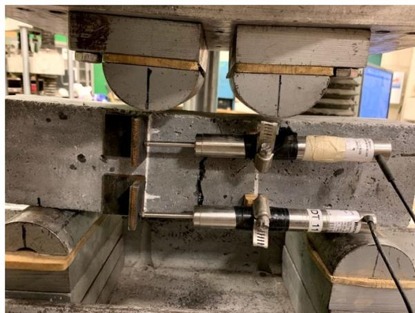
**Figure 10.** UHPC prismatic sample at failure under four-point flexural testing.
