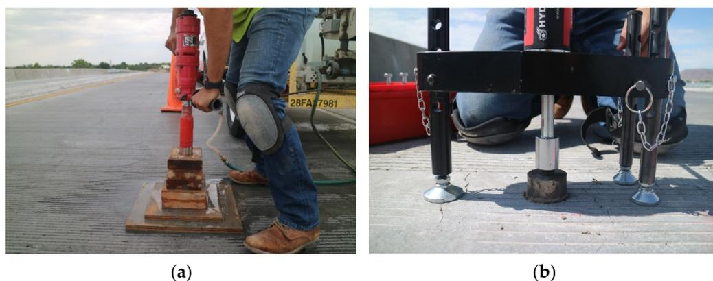
**Figure 11.** Direct tension pull-off testing procedure (a) core drilling and (b) testing set-up.
