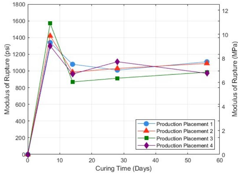
Figure 13. All production placements—modulus of rupture (MOR).
