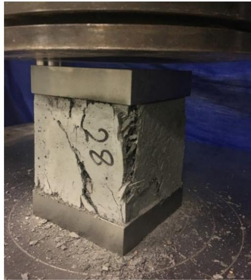
**Figure 9.** UHPC cube sample at failure under compression testing.
