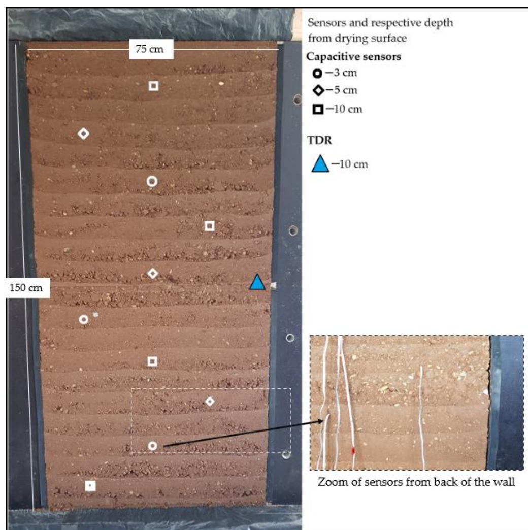
Figure 5. Layout of position of the sensors with their respective depth in the wall. A zoom of sensors final position taken from the back of the wall.
