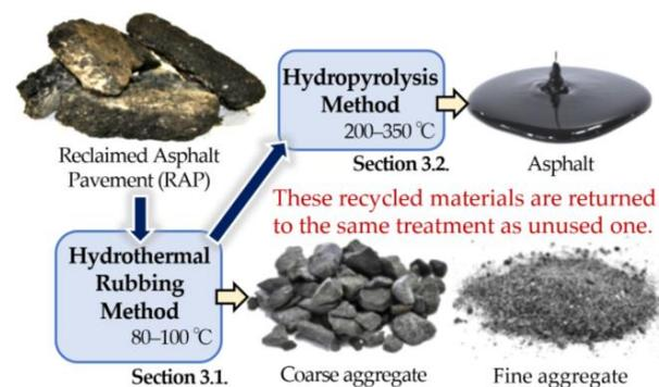
Figure 2. Separate recycling technology.
