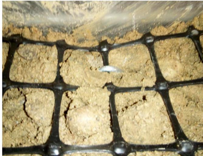
**Figure 15.** Anchoring geogrid using steel peg.
