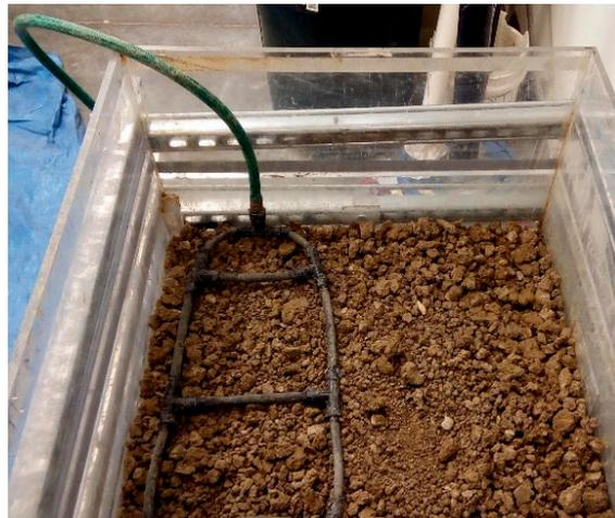
**Figure 5.** Placement of soaker system at the top half of subgrade.
