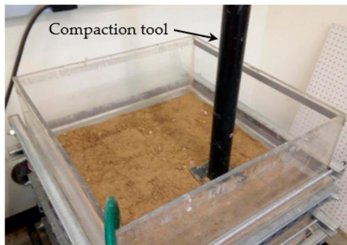
**Figure 4.** Compacted soil and the tool used for compaction.
