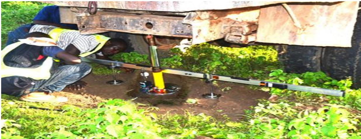
**Figure 3.** Conventional Plate load test.
