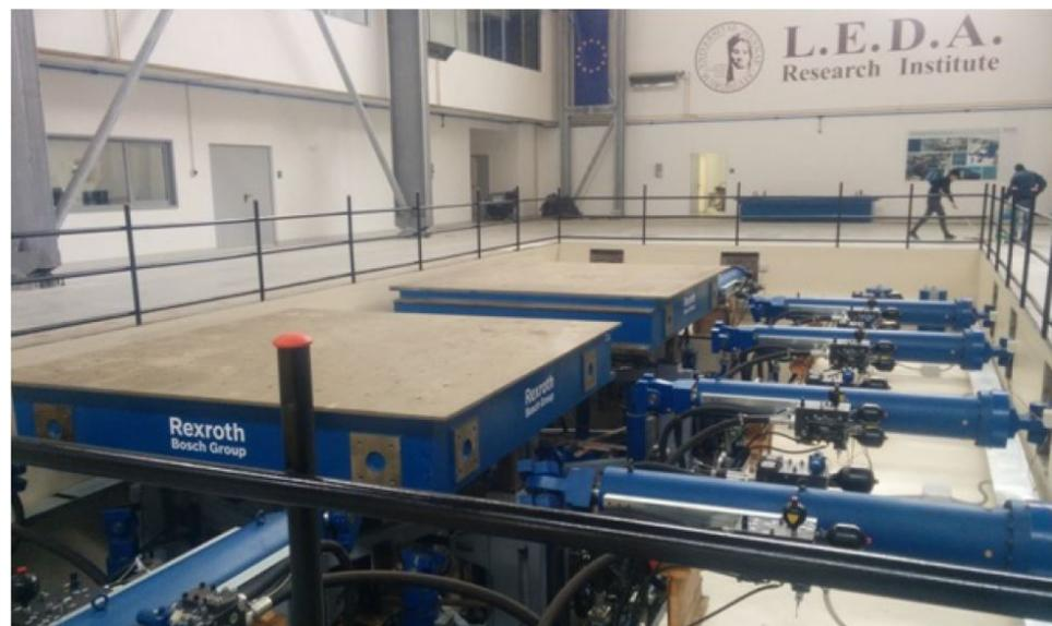
Figure 17. Photographic view of the shaking tables system (From [62]).
