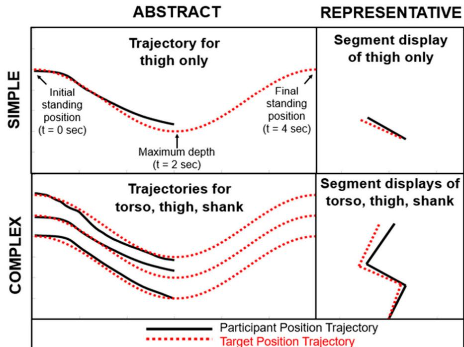
Figure 1. (A) Participant undergoes squat protocol while motion and ground reaction forces are measured. (B) Visual feedback modes defined according to two primary features of complexity ('simple' or 'complex') and representation ('abstract' or 'representative'). Feedback complexity entails tracking one segment (simple) versus three segments (complex). Representation entails observing feedback explicitly as sinusoids (abstract) versus a stick figure (representative).
