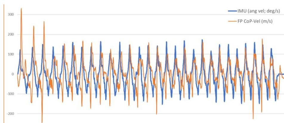
**Figure 3.** Example of raw (example level) inertial measurement unit (IMU, angular velocity, blue line) and force-platform (FP) centre of pressure (CoP, orange line) velocity (m/s) signals from an up-on-the-toes 30 s test (UTT-30).
