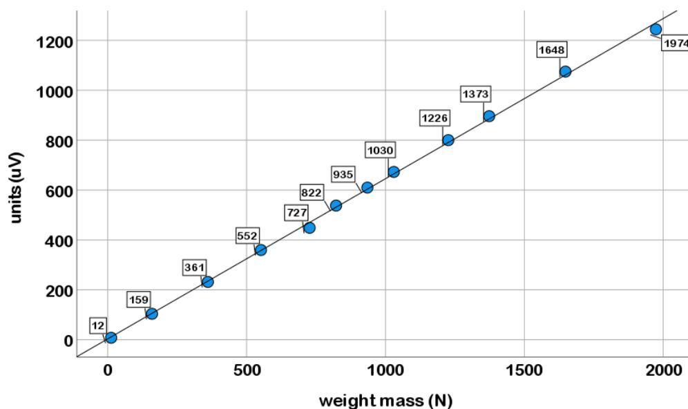
Figure A1. Data dispersion of 170 measures from known weights for the 2-Dynami dynamometer.
