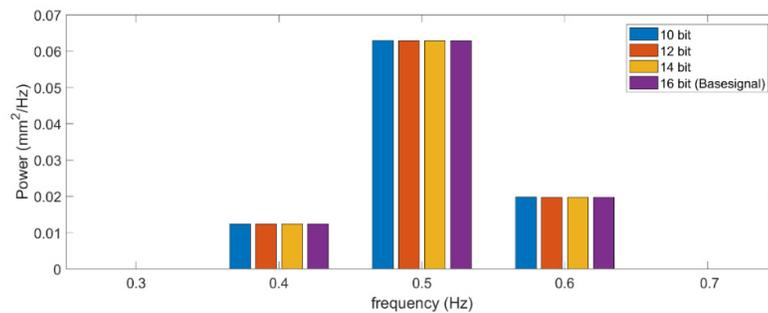
**Figure 3.** Representation of the mean PSD spectrum of the tests with the technical pendulum in different resolutions.
