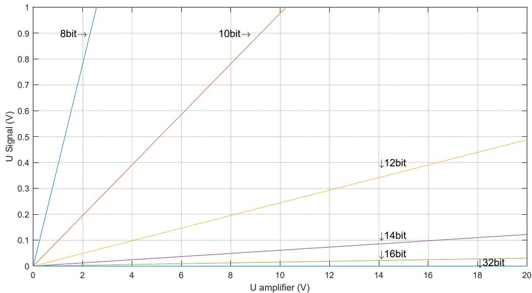
**Figure 5.** Representation of a characteristic diagram for the quality  $Q = 1$  for different resolutions depending on the working range of the A/D converter and the signal amplitude  $U_{sig}$ . The area to the left of the cutoff line describes a  $Q > 1$  to the right of the line  $Q < 1$ .
