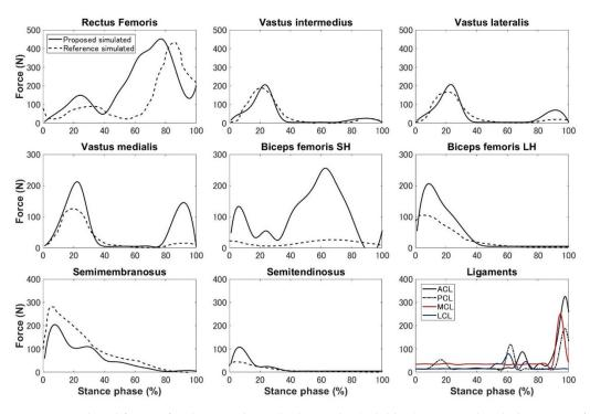
**Figure 5.** Predicted forces of eight major lower limb muscles (solid line) compared with the means of the forces estimated by the OpenSim simulation toolkit for biomechanical analyses [34] averaged across 10 participants (dotted line) and fourpredicted ligament forces during a single stance phase.
