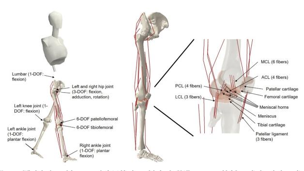
**Figure 2.** Whole-body model, composed of rigid body models for the HAT segment and left lower limb and a lower limb FEMS model. The whole-body model has 22 DOFs. The lower limb FEMS model includes a 12-DOF nature knee joint, muscles and ligaments (displayed in red), cartilages, and a meniscus (displayed in orange).
