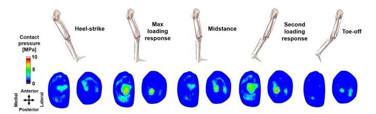
Figure 7. FE analysis result of the contact pressure distribution occurring on the tibial cartilage during the stance phase.
