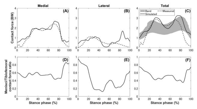
**Figure 8.** Predicted contact forces of the knee joint (solid line) compared with experimental data (Zeighami et al. 2018) (dotted line) and instrumented knee implant data [38] (shaded area): (**A**) medial contact force, (**B**) lateral contact force, (**C**) total contact force on the medial and lateral sides. Predicted ratios of the meniscal contact forces to total tibiofemoral contact forces: (**D**) medial ratio, (**E**) lateral ratio, (**F**) total ratio.
