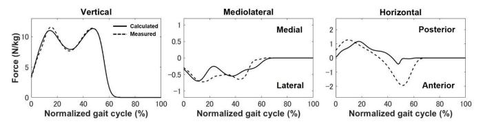
**Figure 3.** Predicted ground reaction forces (solid line) compared with the force plate data (dotted line) for a subject at normal walking speed.
