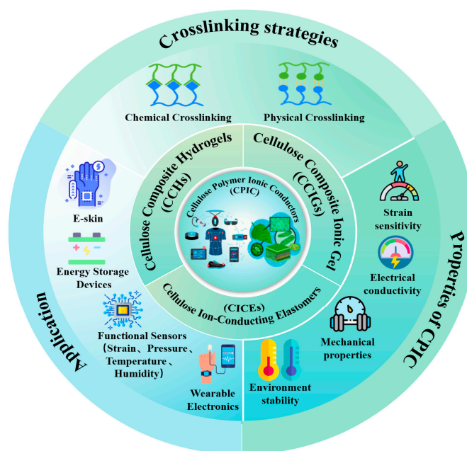
Figure 1. Classification, application areas, crosslinking strategies, and key properties of cellulose-composite polymer ionic conductors.
