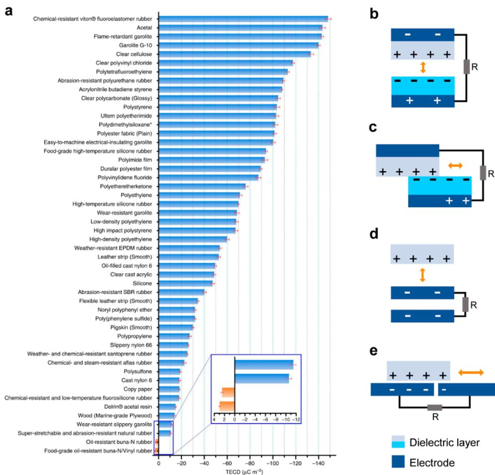
**Figure 1.** Triboelectric series and four fundamental working modes of TENGs. (a) Quantified triboelectric series. Reprinted with permission from ref. [34], Copyright 2019, Springer Nature. (b) Vertical contact-separation mode. (c) Lateral sliding mode. (d) Single-electrode mode. (e) Freestanding triboelectric-layer mode.
