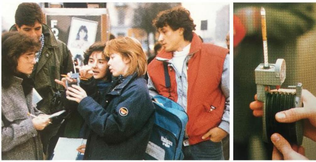
**Figure 4.** Air pollution monitoring: adolescents, there as researchers, measuring the concentrations of polluting gases in the air of the city where they live. They used a hand-held tool (enlarged image on the right), a 100 cc manual Dräger sampling system equipped with single-gas vials.
