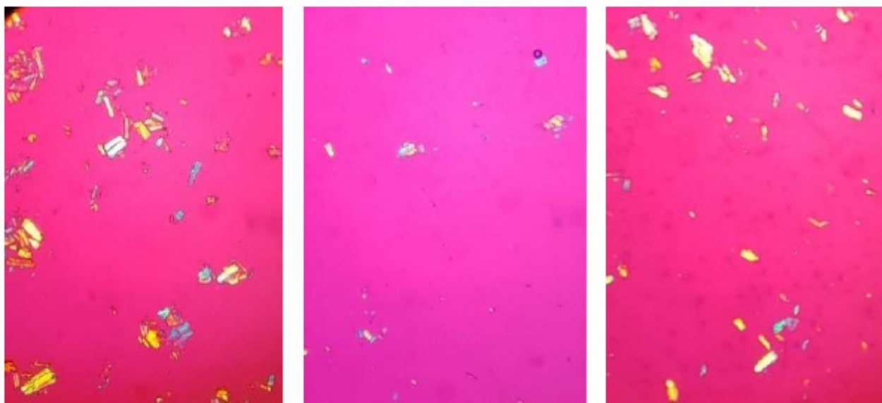
Figure 3. Microscopic analysis of 0.5 mass percent of cellulose in aqueous solution of 4 (from left to right: 10%, 40%, 60%).
