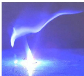
Figure 8. Burn intensity of a film with 2.5 mass % FLG 5 ms after the laser beam was turned off.
