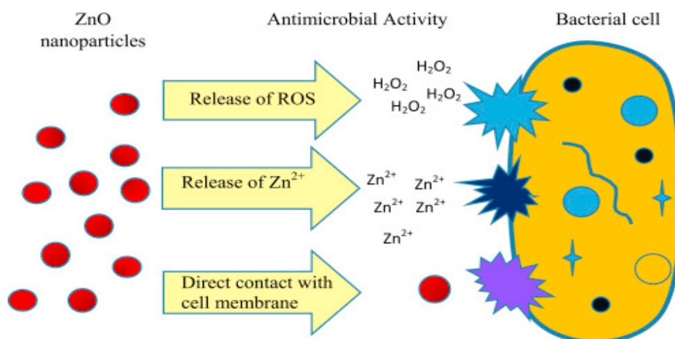
Figure 4. The mechanism of water disinfection by ZnO NPs [183].
