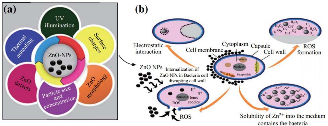
**Figure 1.** (a) An impact of key ZnO NPs parameters on the antibacterial response and (b) correlation between the several potential mechanisms of ZnO NPs antibacterial activity, such as ROS production, Zn<sup>2+</sup> release, internalization of ZnO NPs into bacteria, and electrostatic interactions [34].
