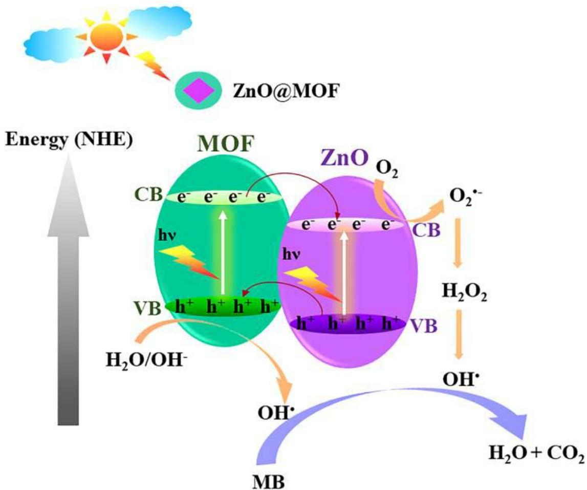
**Figure 2.** Photocatalytic mechanism of ZnO@MOF-46(Zn). Proposed reaction mechanism over ZnO@MOF-46(Zn) for photodegradation [82].
