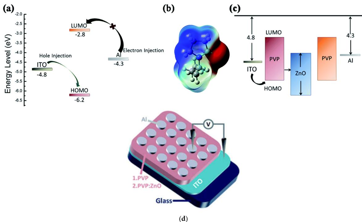
**Figure 5.** (a) Energy level diagram of the devices that are based on PVP. (b) The electrostatic potential (ESP) of the molecule as determined using DFT. (c) Illustration of the energy bands of the ITO/PVP:ZnO/Al device. (d) Schematic structure of resistive random-access memory (RRAM) device based on polyvinylpyrrolidone (PVP) and PVP:PVP:zinc oxide nanoparticle (ZnO NP) active layers [217].
