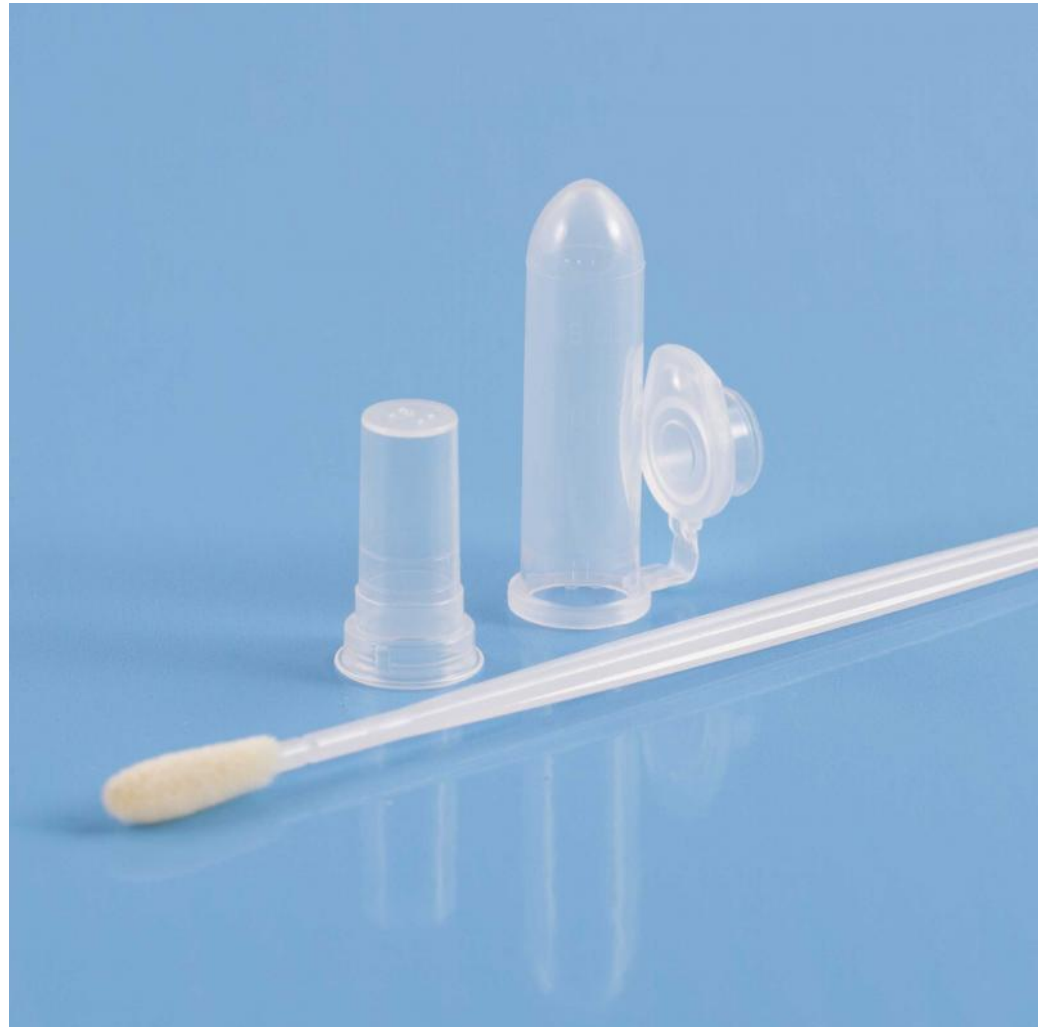
Figure 7. The NAO spin basket from copan italia is a special plastic semipermeable basket that allows recovery of nucleic acids from specimens, including swab samples, into the sample tube. From: https://www.omnia-health.com/product/nao%20basket (accessed on 13 December 2023).
